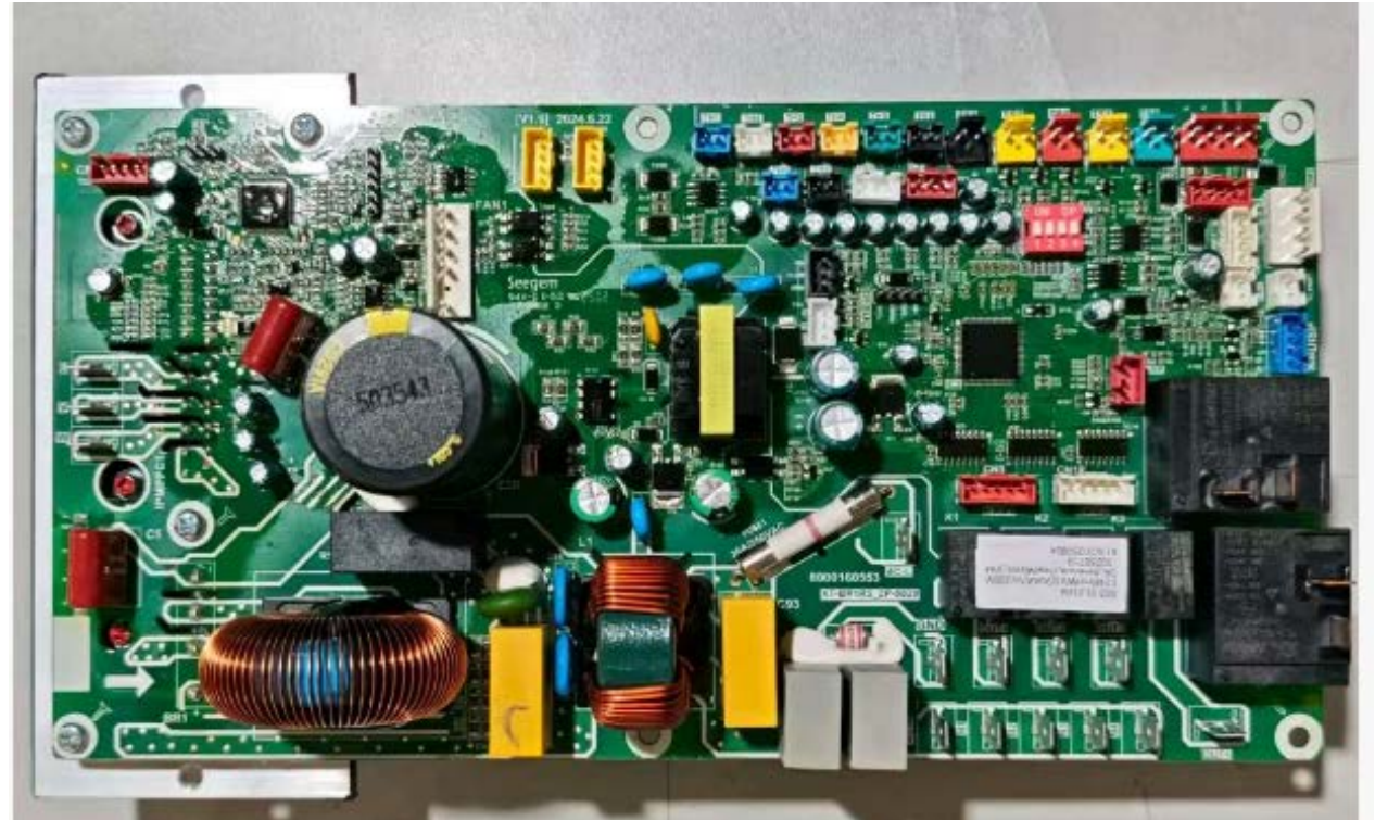
PCB of the heat pump
