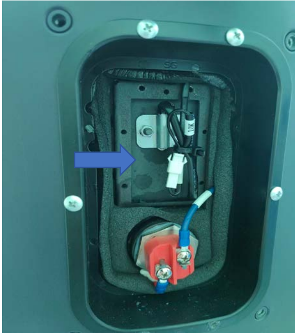
Temperature probe in the middle of the water tank
